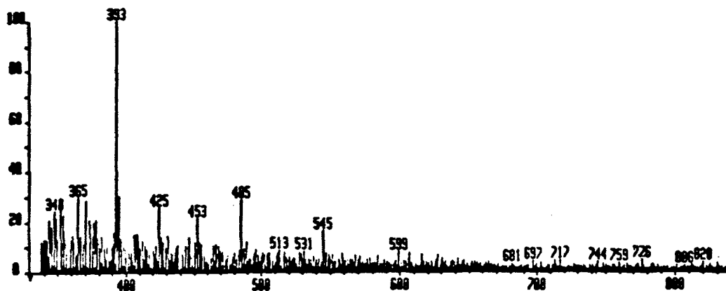
Figure 10 Mass spectra of SMAA oligomer.
